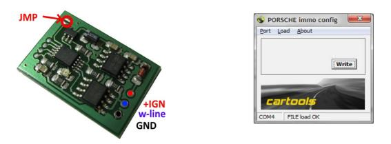
**NOTE**: before loading dump into configurator software, attach emulator first and make "test write" (write any trash into emulator) to enable FILE LOAD option.
